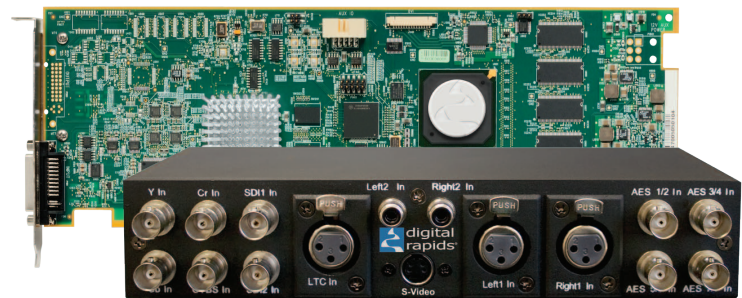
Flux-6550 with optional breakout box
